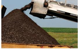
plant or a portable plant. The recycled material can be replaced on the original pavement or transported to a different road.
